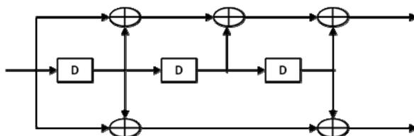
Figure 7-14: Convolutional Code with constraint length 4
