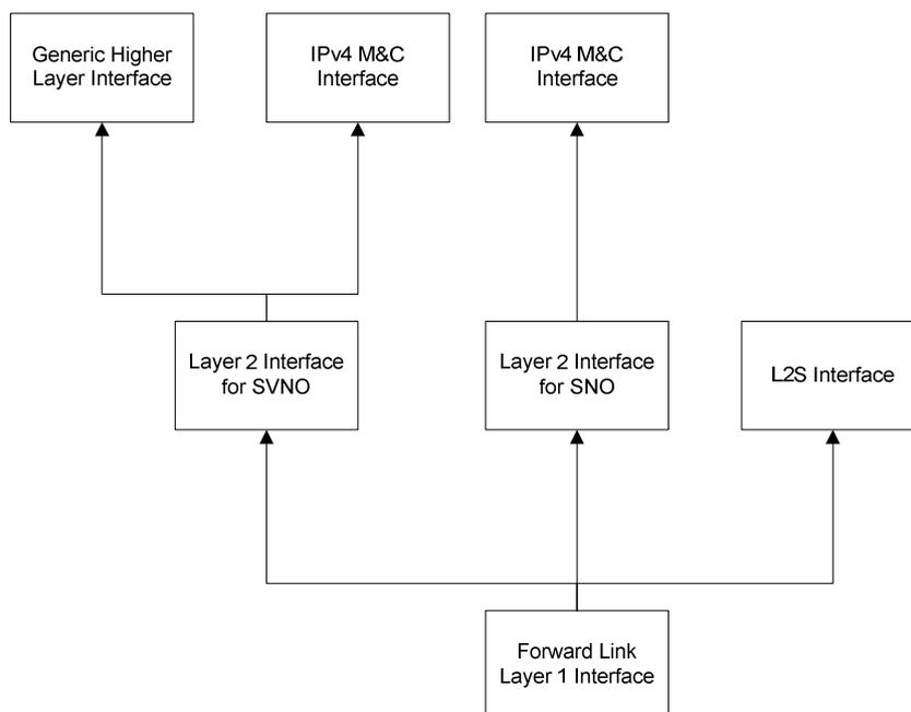
**Figure 4-5: Forward Link Interfaces at an RCST**
