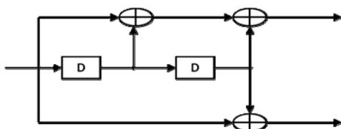
Figure 7-13: Convolutional code with constraint length 3
