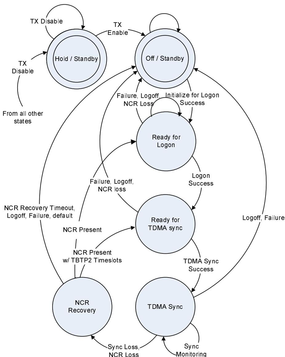
**Figure 9-1: RCST State Diagram for MF-TDMA Operation**
