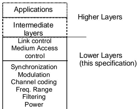
**Figure 4-1: Identification of the Lower Layers**
