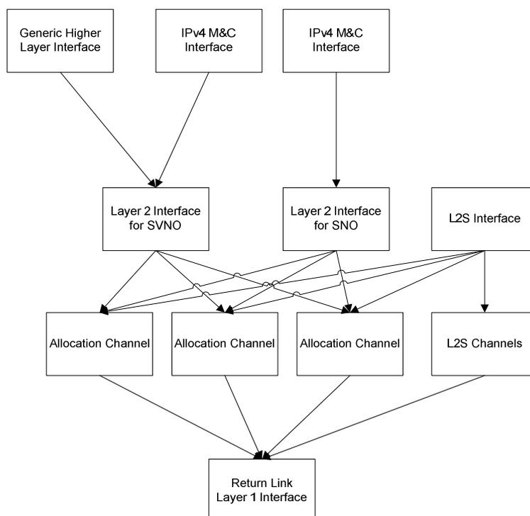
**Figure 4-6: Return Link Interfaces at an RCST**
