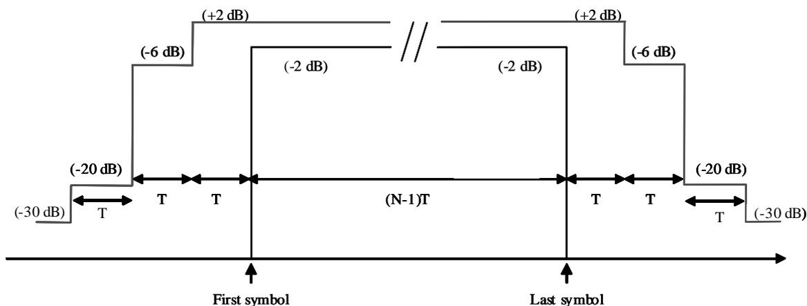
**Figure 7-21: Burst power envelope mask for TC-LM bursts**
