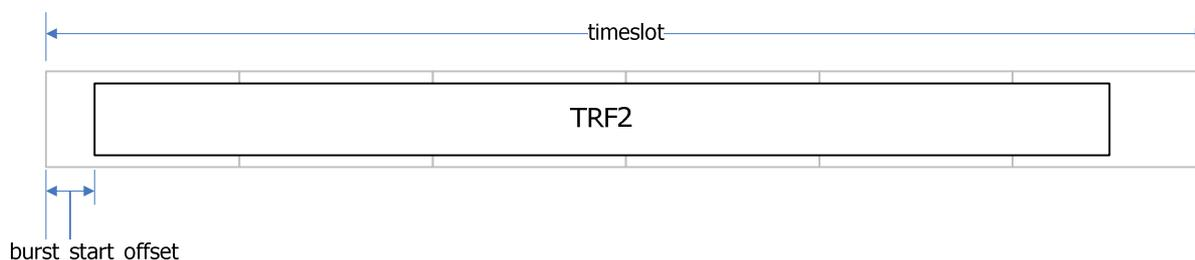
**Figure 7-27: Example of a Burst in a Timeslot Built from 6 BTUs**
