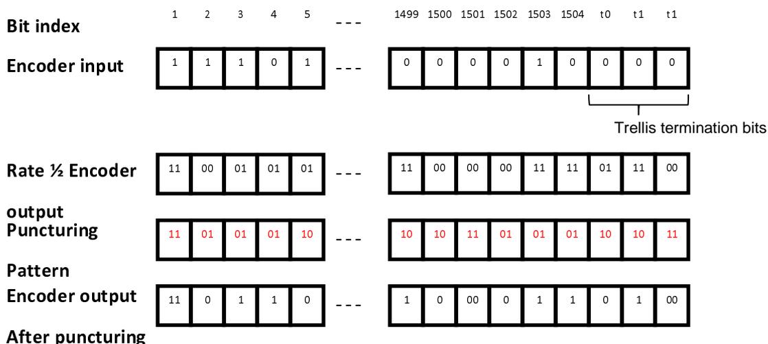
Figure 7-15: Puncturing process for rate 6/7, K=4 convolutional code
