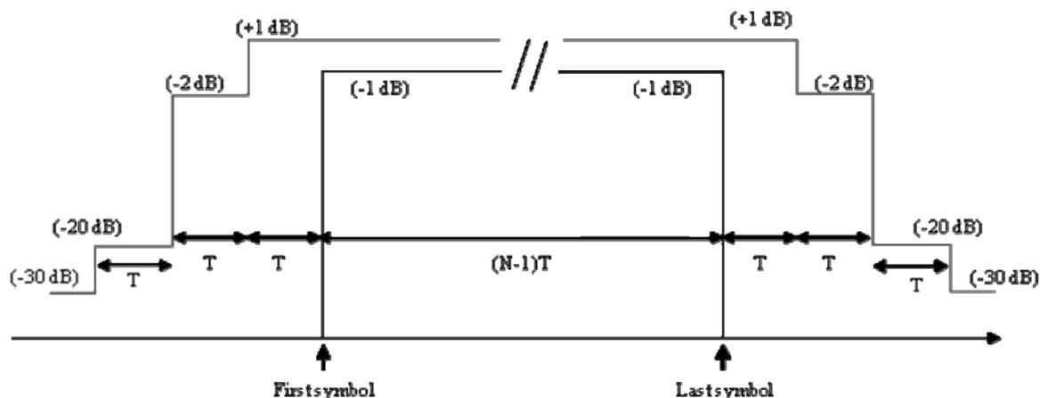
**Figure 7-22: Burst power envelope mask for CC-CPM bursts**
